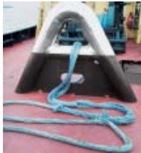
Strop to main line connection.
