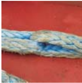
Eye-to-eye single leg connection.
