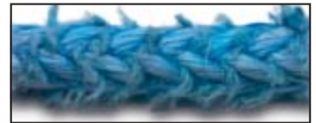
FIG. 3 Severely abraded rope
