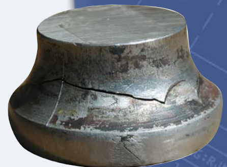
Transverse crack in Rod Head
