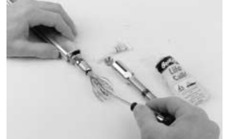
Norseman/Sta-Lok fitting being assembled.
